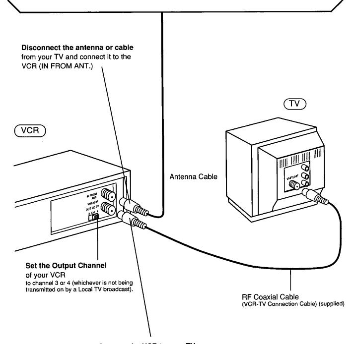
Connect the VCR to your TV with the RF Coaxial Cable (OUT TO TV).
